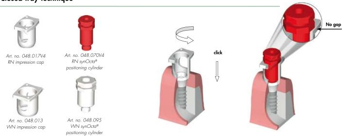
After removing the healing cap with an SCS screwdriver, clean both the shoulder and the internal configuration of the implant of blood and tissue residue prior to the impression procedure. Push the impression cap onto the implant shoulder until it clicks into place. Gently turn the impression cap to ensure that it is securely seated. When the cap is properly engaged, it can be rotated on the implant.
